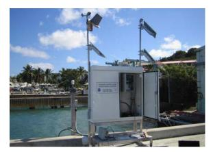
Figure 8. Coastal water-level station
