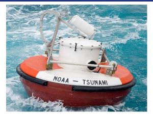
Figure 7. DART system buoy
