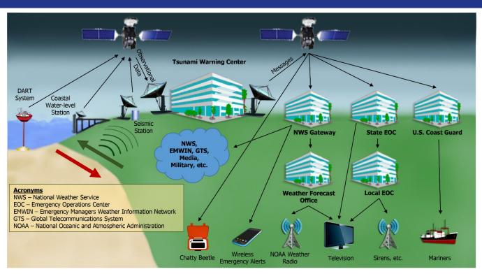
Figure 9. U.S. Tsunami Warning System diagram. Source: NOAA/National Weather Service
