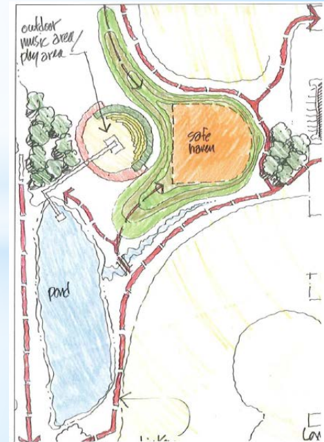
Illustration 10: Elementary School Site Berm Structure (a) and (b). The orange color-dashed area highlights the safe zone imbedded into the school berm.
